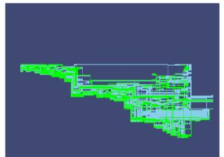
Fig (9) MIMO decoder after placement / routing on Xilinx Virtex 4
